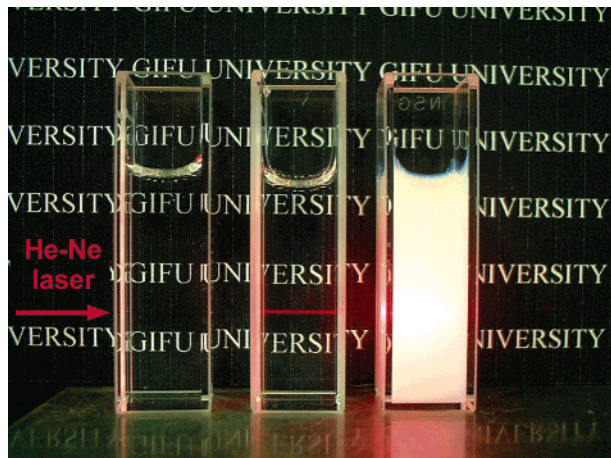
Figure 1. Photograph of the solutions of (a) distilled water, (b) 1 M TIP-TMAOH ( R = 0.4 ) and (c) 0.5 M crystalline anatase suspension (STS-01).
